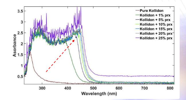
*In-line* UV-Vis spectra from Piroxicam / polymer extrudates
